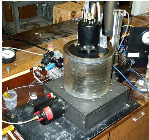
Figure 2: UC Berkeley bi-directional Simple Shear Device
